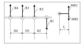
**Fig. 11.** Scheme for calculating the forces acting in the external support at the points of its connection with the rods, where R1 and R2 are the forces acting on the rod; R3, R4 are the reactions in the supports transmitted to the proximal fragment, MR1 and MR2 are the torques; H2 is the distance between the rods on the distal "fragment", H3 is the distance between the second and third rods close to the "fracture", H4 is the distance between the rods on the rods on the proximal "fragment"
