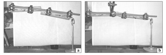
**Fig. 8.** The magnitude of the distal "fragment" displacement at maximum load of the model with the use of the "Orthofix" device, provided that all rods are located in the frontal plane (a) and during the insertion of one rod, which is in the proximal fragment in a plane that is at 45° to the frontal plane (b) (structure parameters 9, 14 in Table 1)
