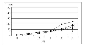
**Fig. 5.** Linear displacements during stepwise loading of the models with geometric parameters indicated under numbers 5 and 6 of the table using the devices "HB ORTHO" (1 - 3 rods,100 mm; 2 - 3 rods, 100 mm) and "Orthofix" (3 - 3 rods, 100 mm; 4 - 3 rods, 100 mm)
