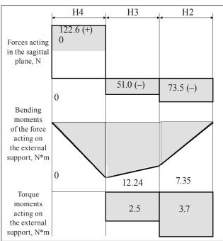
Fig. 12. External support load diagrams
