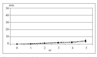
**Fig. 6.** Linear displacements during stepwise loading of the models with geometric parameters indicated under numbers 7 and 8 of the table using the devices "HB ORTHO" and "Orthofix"
