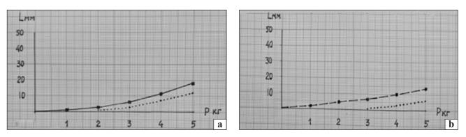
Fig. 6. Graphs showing linear displacements of the ends of the "fragments" during stepwise loading of the models and using the devices "HB ORTHO" (a) and "Orthofix" (b)
