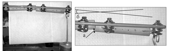
**Fig. 2.** General view of the model under load and deformation: a — linear displacement of the distal "fragment"; b — angular displacement of the distal "fragment"
