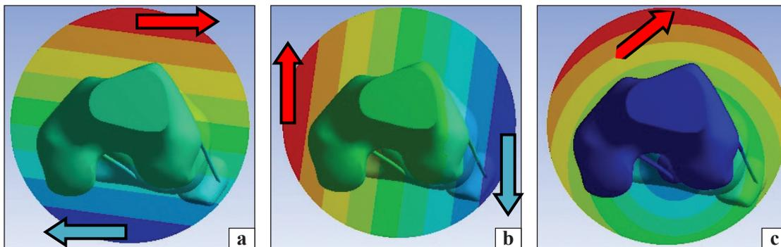
**Fig. 7.** Distribution of displacement fields in the calculation models (top view): along the  $x$ -axis (a),  $y$ -axis (b) and full displacement  $d$  (c). Arrows show the points of origin and directions of the specified maximum displacements
