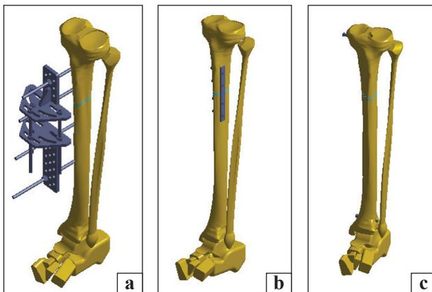
**Fig. 1.** Models of tibial fracture in the upper third with osteosynthesis: a) EFD; b) bone plate; c) intramedullary rod
