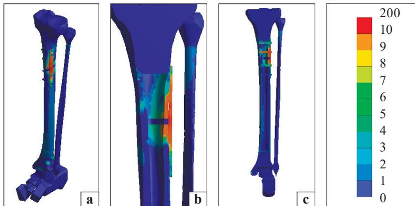
**Fig. 4.** Pattern of stress distribution in the lower leg model with a fracture of the tibia in the upper third (osteosynthesis with a bone plate) under a torsional load of 7.0 Nm: a) general view; b) fracture zone; c) intersection of the tibia
