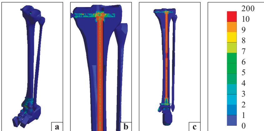
**Fig. 5.** Pattern of stress distribution in the lower leg model with a fracture of the tibia in the upper third and osteosynthesis with an intramedullary rod under a torsional load of 7.0 Nm: a) general view; b) fracture zone; c) intersection of the tibia
