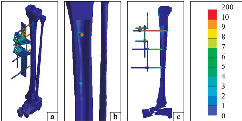
**Fig. 3.** Pattern of stress distribution in the lower leg model with a fracture of the tibia in the upper third (osteosynthesis with an EFD) under a torsional load of 7.0 Nm: a) general view; b) fracture zone; c) intersection of the tibia
