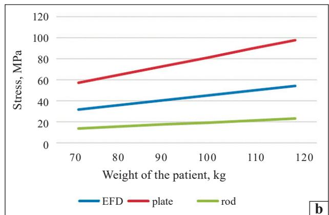
**Fig. 10.** Graphs of the dependence of stress values on the weight of the patient in the elements of metal structures (a) and around the fixing screws and rods (b) in the tibia after its fracture in the upper third and various types of osteosynthesis
