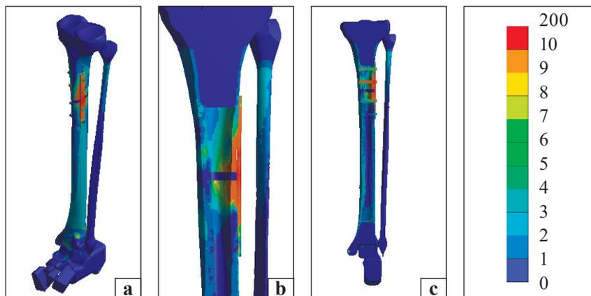
**Fig. 7.** SSS in the lower leg model with a fracture of the tibia in the upper third under a torsional load of 12.0 Nm, osteosynthesis with a bone plate: a) general view; b) fracture zone; c) intersection of the tibia
