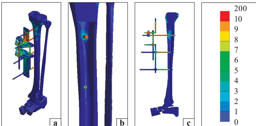
**Fig. 6.** Pattern of stress distribution in the lower leg model with a fracture of the tibia in the upper third under a torsional load of 12.0 Nm, EFD osteosynthesis: a) general view; b) fracture zone; c) intersection of the tibia
