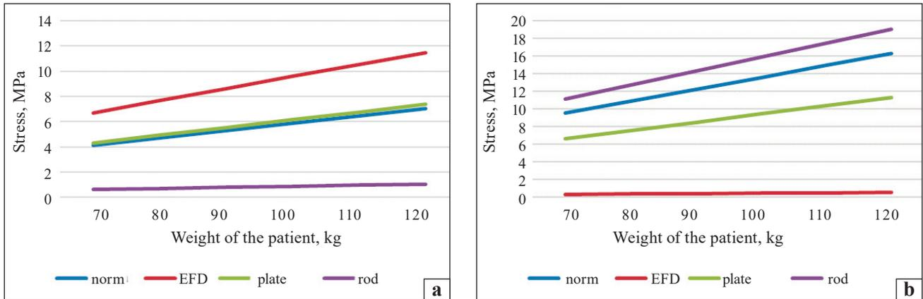
**Fig. 9.** Graphs of the dependence of stress values on the patient's weight in models of the tibia with fractures in its upper third and various types of osteosynthesis: proximal (a) and distal (b) fragments; fracture zone (c)
