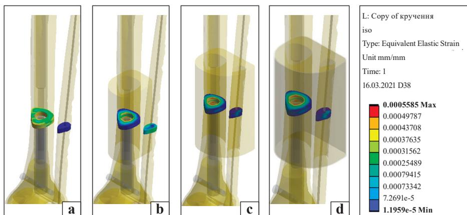
**Fig. 4.** Relative deformations of the bone regenerate in the model of the lower leg with pseudoarthrosis of both bones in the lower third, compressive load. Rotationally stable rod. Osteosynthesis: a) rod and spoke; b) rod and spoke + bone graft in the form of a block on the tibia; c) rod and spoke + bone graft on both bones; d) rod and spoke + bone graft on both bones, covered with a titanium mesh
