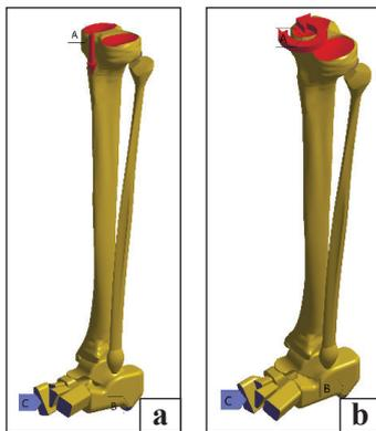
**Fig. 2.** Models load schemes: a) vertical axial compression; b) torsion
