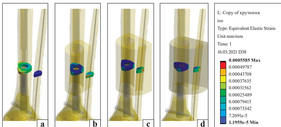
**Fig. 6.** Relative deformations of the bone regenerate in the model of the lower leg with pseudarthrosis of both bones in the lower third, torsional load. Rotationally stable rod. Osteosynthesis: a) rod and spoke; b) rod and spoke + bone graft in the form of a block on the tibia; c) rod and spoke + bone graft on both bones; d) rod and spoke + bone graft on both bones, covered with a titanium mesh
