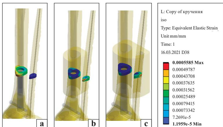
**Fig. 5.** Relative deformations of the bone regenerate in the model of the lower leg with pseudarthrosis of both bones in the lower third under the influence of torsional load. Fassier-Duval rod. Osteosynthesis: a) rod and spoke; b) rod and spoke + bone graft in the form of a block on the tibia; c) rod and spoke + bone graft on both bones
