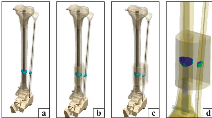
**Fig. 1.** Models of the lower leg with a bone fracture in the lower third. Osteosynthesis: a) rod and spoke; b) rod and spoke + bone graft in the form of a block on the tibia; c) rod and spoke + bone graft on both bones; d) rod and spoke + bone graft on both bones, covered with titanium mesh
