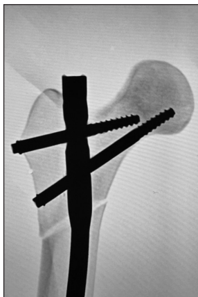
Fig. 3. The radiological image demonstrates the fixation of a FIN-3 following the anatomical reduction of a reverse oblique subtrochanteric fracture model
